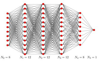
Figure 1.1: Illustration of a multi-layer perceptron with 5 layers. The red dots correspond to the neurons.
